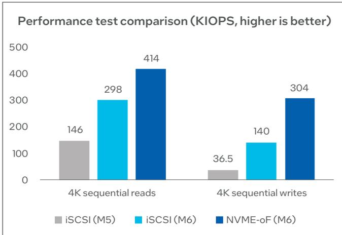
Figure 6. Comparison of 4K read/write performance between iSCSI and NVMe-oF storage protocols on M5/M6 platforms<sup>3</sup>
