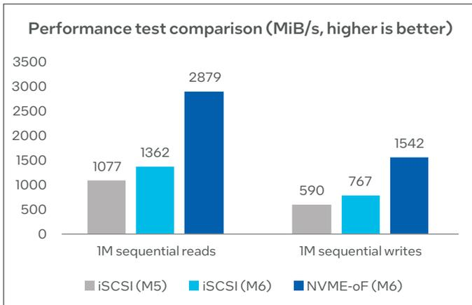
Figure 7. Comparison of 1MB read/write bandwidth between iSCSI and NVMe-oF storage protocols on M5/M6 platforms<sup>4</sup>
