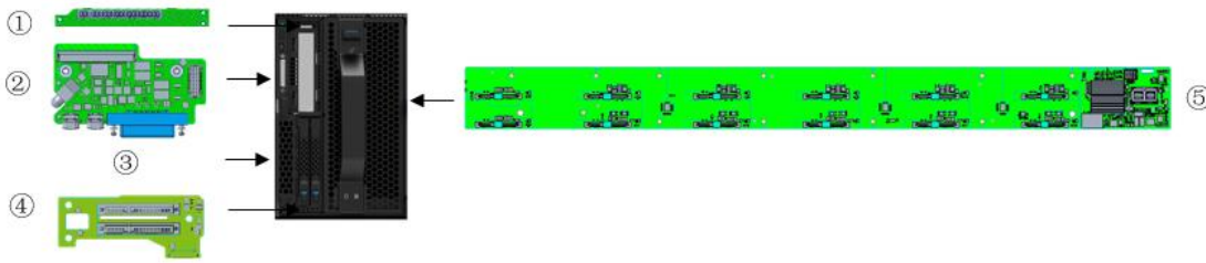
Figure 41 Front panel card view of the 2SFF 1LP system on the NF5484M5 node
