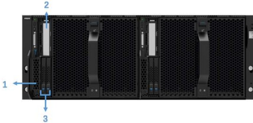
Figure 20 Front panel of the 2SSD 1LP system on the NS5482M5 node
