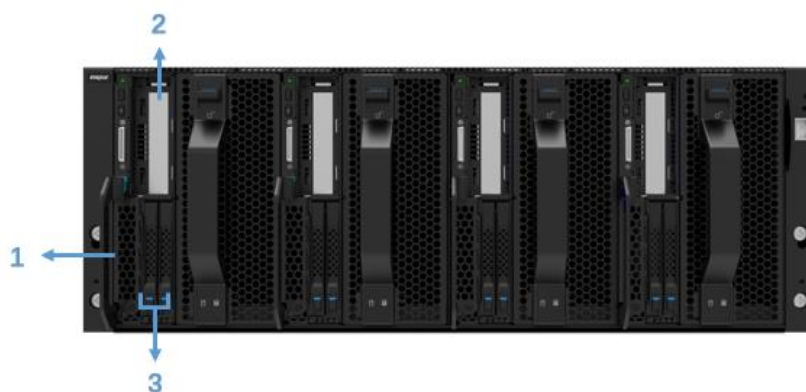
Figure 14 Front panel of the 2SFF 1LP system on the NS5484M5 node
